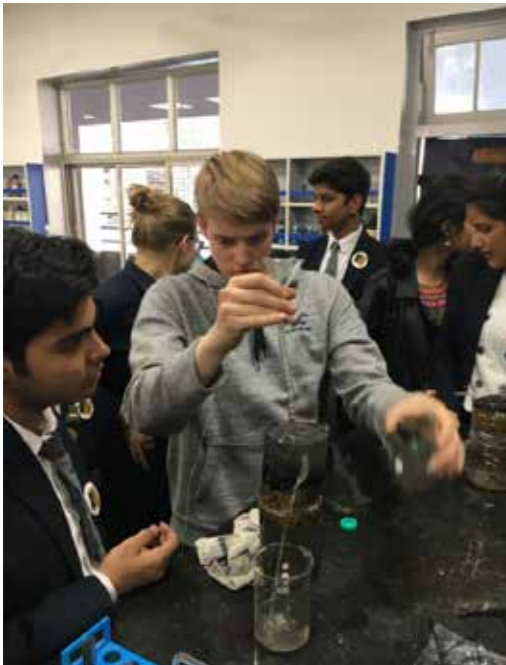
Fig. 10.2: Model experiment for the purification of water through different layers arranged in two 2-L-bottles (photo: Steinmetz, 2019).
